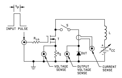
Input pulse Rin = 50 ohms, 1 watt  $V_G = 10 \text{ Volts}$  $R_S = 0.1$  ohms, 1 watt  $R_G = 50 \text{ ohms}$
