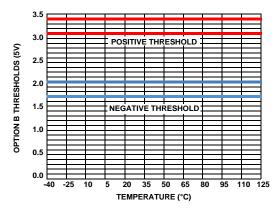
FIGURE 2. TEMPERATURE STABLE LOGIC THRESHOLDS
