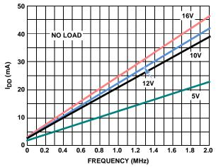
FIGURE 12. I<sub>DD</sub> vs FREQUENCY (+25°C)
