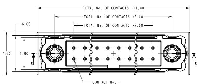
M80-5T2<u>XXXX</u>BI-<u>XX-XXX-XX-XXX</u> TOTAL No. OF CONTACTS-06, 10, 14, 20, 26 FINISH CODE-05 - ALL OVER GOLD 22 - GOLD ON CONTACT AREA / TIN/LEAD ON TAIL 42 - GOLD ON CONTACT AREA / 100% TIN OVER NICKEL ON TAIL NUMBER OF SPECIAL CONTACTS -X'S CAN BE DISPLAYED AS TRAILING ZEROS OR LEFT BLANK SEE EXAMPLE ORDER CODES FOR EXPLANATION.
