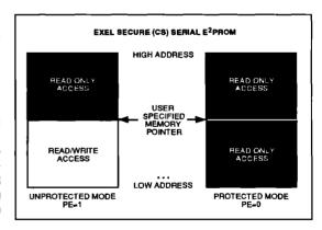
The figure above shows the status of the memory array regions as defined by the pointer address and the state of the program enable (PE) pin. In the first case, programming operations are enabled through the application of a logic "1" to the PE control pin. All memory locations beneath that of the pointer address are available for data changes. All memory locations at or above the pointer address are protected against data alteration and serve as read only memory.
