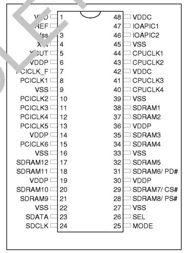
PS# =: PCI\_STOP, CS# = CPU\_STOP,
