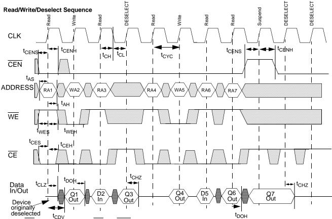
WE is the combination of  $\overline{WE}$  and  $\overline{BWS}_X(x=a,b,c,d)$  to define a write cycle (see Write Cycle Description table).  $\overline{CE}$  is the combination of  $\overline{CE}_1$ ,  $\overline{CE}_2$ , and  $\overline{CE}_3$ . All chip selects need to be active in order to select the device. Any chip select can deselect the device. RAx stands for Read Address X, WA stands for Write Address X, Dx stands for Data-in X, Qx stands for Data-out X.
