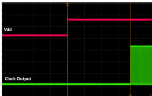
Figure 17. Startup Waveform vs. Vdd
