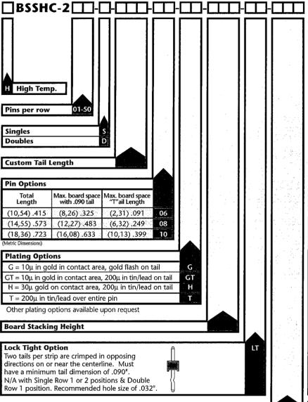
**EXAMPLE:** If you want a 20 position, single position elevated board socket with an elevated height of .400 and a tail of .114 order a BSSHC-220-S-114-08-T-400.
