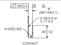
SCALE 1.5: CRITICAL 1 DIMMENSION MUST BE VERIFIED AT BEGINNING, MIDDLE, AND END OF EACH LOT
