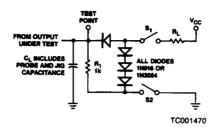
Note: For standard totem-pole outputs, remove R1; S1 and S2 closed.
