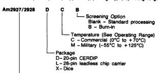
Device type Quad 3-state Bus Transceivers
