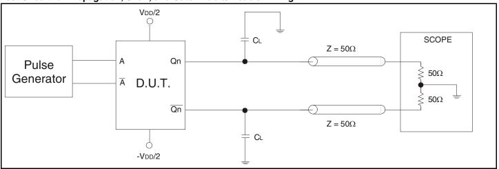
**Table 6B. Differential Input Test Conditions**
