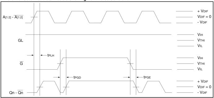
NOTE 1: As shown, it is possible to generate runt pulses on gate disable and enable of the outputs. It is the user's responsibility to time the G signal to avoid this problem.
