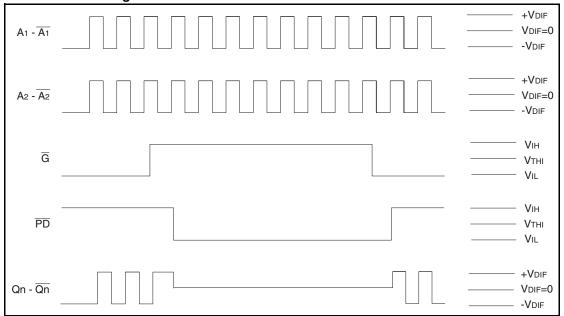
NOTE 1: It is recommended that outputs be disabled before entering power-down mode. It is also recommended that the outputs remain disabled until the device completes power-up after asserting  $\overline{PD}$ .
