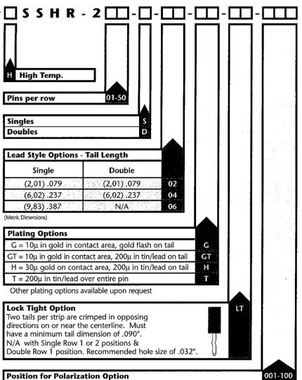
**EXAMPLE:** To order a right angle single row 50 position socket strip with a tail length of .079" and tin plating, the part number is SSHR-250-5-02-T.
