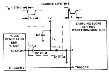
The value of the reverse current (IR) is approximately 6 mA and the forward current (IF) is 1.7 IR. The input pulse is provided by a pulse generator having a rise time of less than one nanosecond. Lifetime is measured between 50% and 90% points of output pulse as shown.
