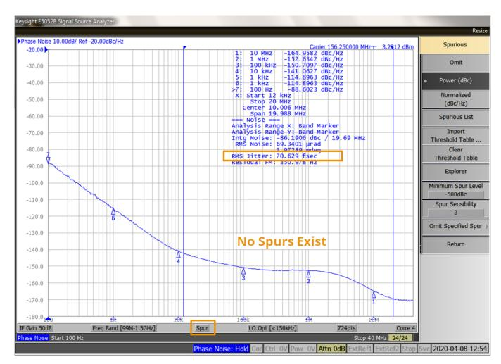
Figure 3. Phase Noise Plot of 3.3 V 156.25 MHz LVPECL Device at 25°C
