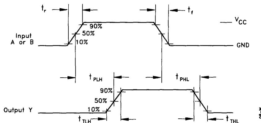
Input and Output threshold voltage, V<sub>T</sub>=50% V<sub>CC</sub> for HC; 1.3V for HCT
