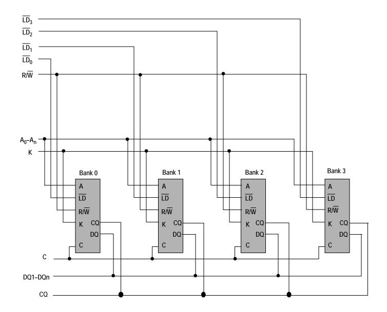
Note: For simplicity  $\overline{\text{BWn}}$  (or  $\overline{\text{NWn}}$ ),  $\overline{\text{K}}$ , and  $\overline{\text{C}}$  are not shown.
