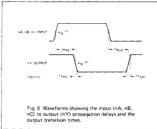
Fig. 6 Waveforms showing the input (nA, nB, nC) to output (nY) propagation delays and the output transition times.
