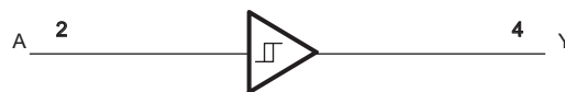
Figure 5. Logic Diagram (Positive Logic) (DBV, DCK, DPW, DRL, DRT, DRY, and YZP Packages)
