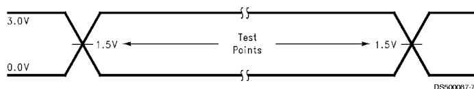
AC testing inputs are driven at 3.0 V for a logic "1" and 0.0 V for a logic "0." Timing measurements are made at 1.5 V for input and output transitions in both directions.
