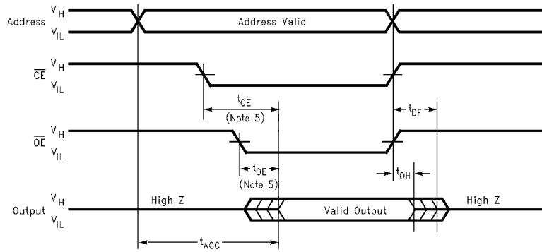
Note 5:  $\overline{OE}$  may be delayed up to  $t_{CE} - t_{OE}$  after the falling edge of  $\overline{CE}$  without impact on  $t_{CE}$ .
