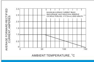
Fig.1 FORWARD CURRENT DERATING CURVE
