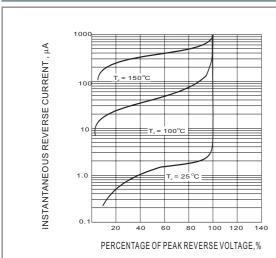
Fig.5- TYPICAL REVERSE CHARACTERISTIC
