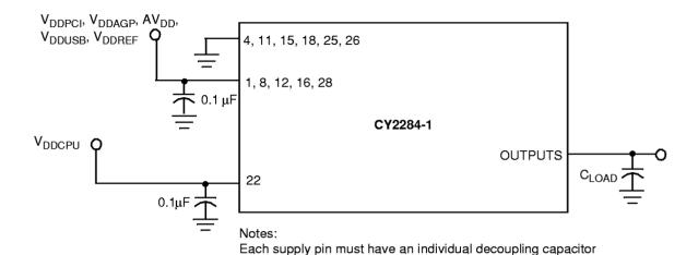
All capacitors must be placed as close to the pins as is possible.
