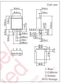
Note) Self-supported type package is also prepared. Internal Connection
