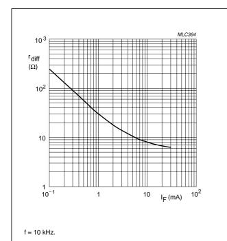
Fig.4 Differential forward resistance as a function
