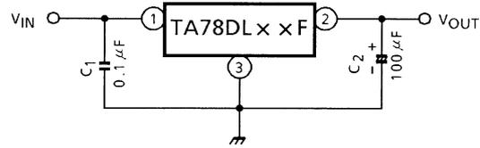
The capacitors  $C_{IN}/C_{OUT}$  must be guaranteed to operate within the temperature range in which the regulator operates correctly.
