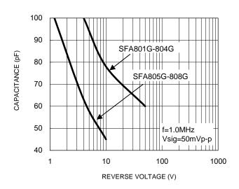
Fig.2 Typical Junction Capacitance
