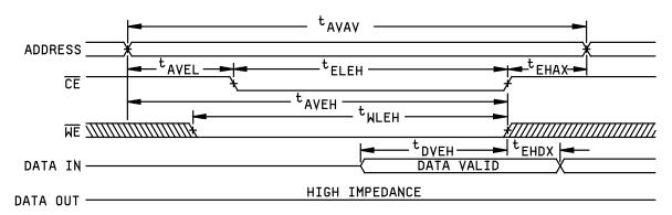
NOTE:  $\overline{\text{CE}}$  or  $\overline{\text{WE}}$  must be  $\geq V_{\text{IH}}$  during address transitions.
