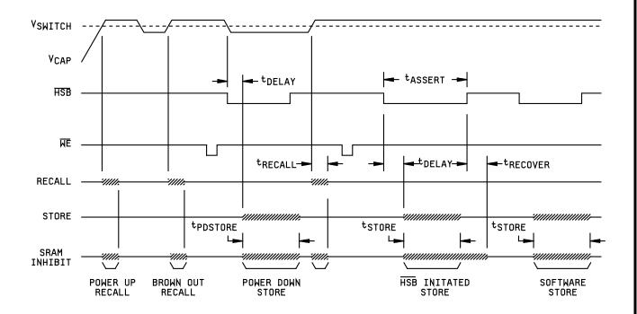
NOTE: RECALL and STORE indicate operations performed within the nvSRAM. These operations are transparent to the user except where SRAM INHIBIT indicates that the SRAM cannot be accessed (outputs are tri-state, inputs are disabled).
