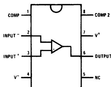
\*Package is connected to Pin 4 (V<sup>-</sup>)
