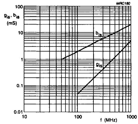
$V_{DS} = 15$  V;  $V_{GS} = 0$ ;  $T_{amb} = 25$  °C; typical values.
