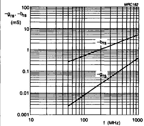
$V_{DS} = 15$  V;  $V_{GS} = 0$ ;  $T_{amb} = 25$  °C; typical values.
