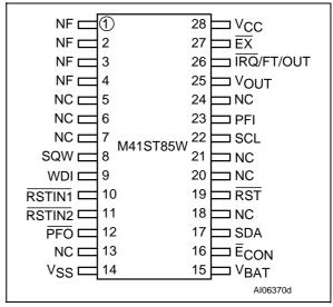
Note: No Function (NF) pins should be tied to VSS. Pins 1, 2, 3, and 4 are internally shorted together.
