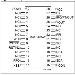
Figure 5. 28-pin, 300mil SOIC (MX) Connections
