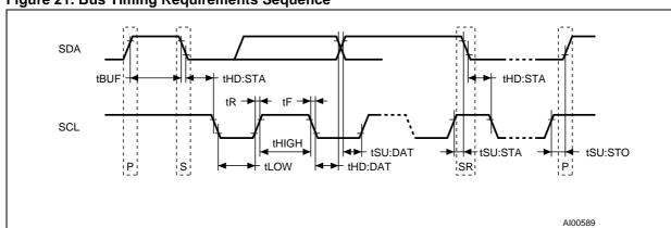
Figure 21. Bus Timing Requirements Sequence
