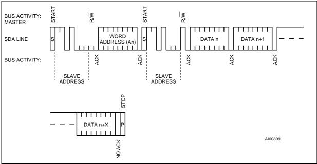
Figure 13. Alternate READ Mode Sequence
