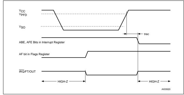
Figure 18. Back-Up Mode Alarm Waveform
