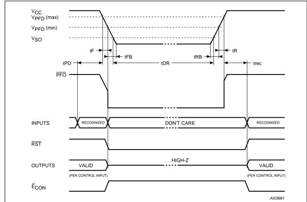
Figure 22. Power Down/Up Mode AC Waveforms
