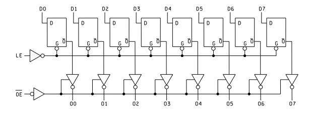
FIGURE 3. Logic diagram.
