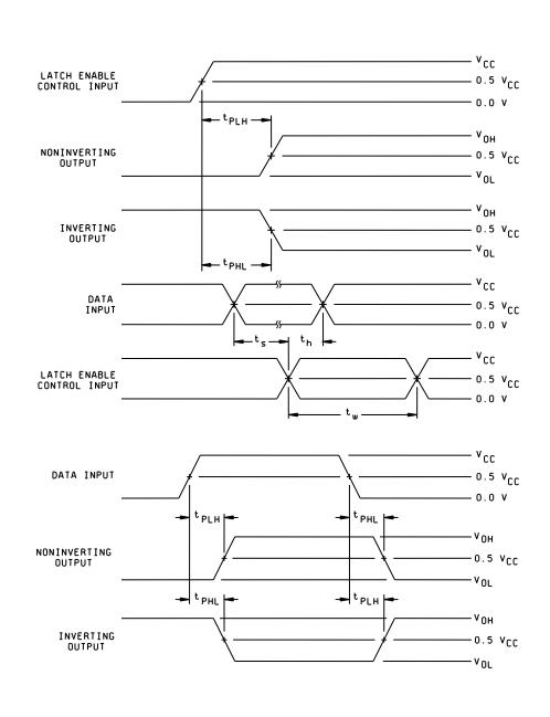
FIGURE 5. Switching waveforms and test circuit.
