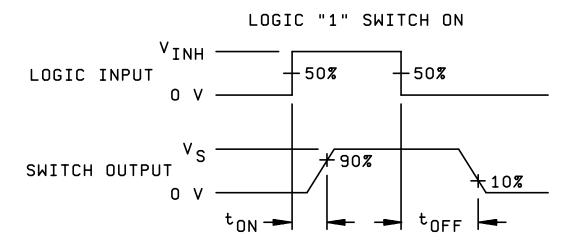
NOTE: For device types 01 and 03,  $V_{INH}$  = +4 V. For device type 02,  $V_{INH}$  = +15 V.
