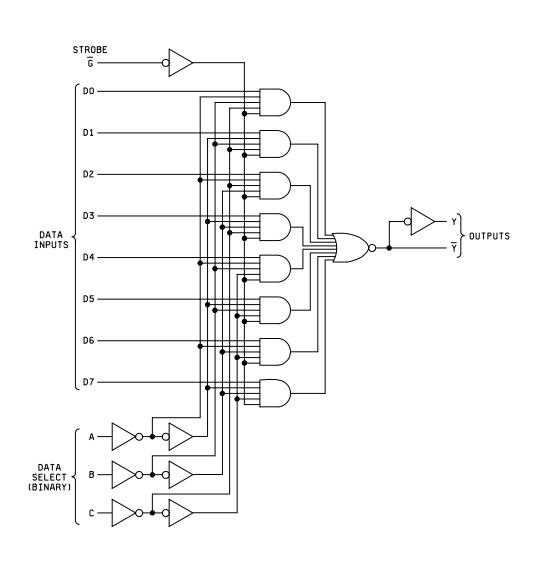
FIGURE 3. Logic diagram.
