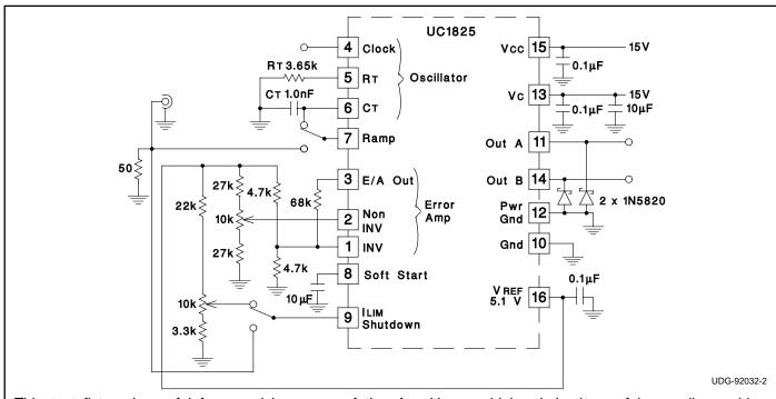
This test fixture is useful for exercising many of the As with any wideband circuit, careful grounding and by-UC1825's functions and measuring their specifications.
