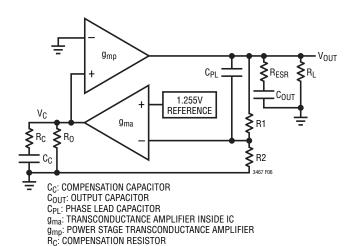
RL: OUTPUT RESISTANCE DEFINED AS VOUT DIVIDED BY ILOAD(MAX) R<sub>O</sub>: OUTPUT RESISTANCE OF g<sub>ma</sub> R1, R2: FEEDBACK RESISTOR DIVIDER NETWORK
