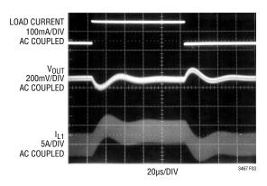
Figure 3. Transient Response of Figure 8's Step-Up Converter without Phase Lead Capacitor
