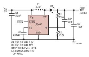
Figure 8. 5V to 12V, 270mA Step-Up Converter
