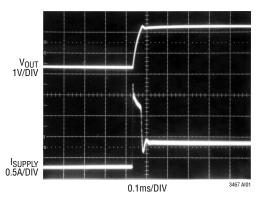
Supply Current of Figure 2 During Start-Up with a 47nF Soft-Start Capacitor
