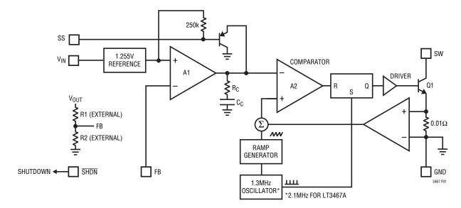
Figure 1. Block Diagram
