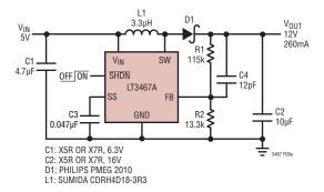
Figure 9. 5V to 12V, 260mA Step-Up Converter
