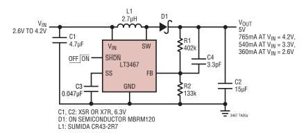
Figure 2. Single Li-lon Cell to 5V Boost Converter (Same as 1st Page Application)
