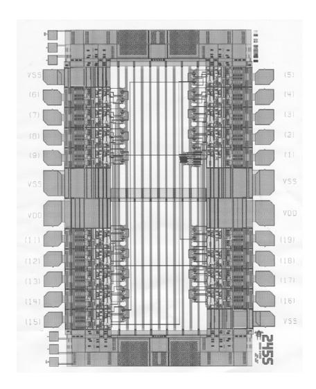
NOTE: Pad numbers reflect terminal numbers when placed in case outlines R and X (see figure 1).
