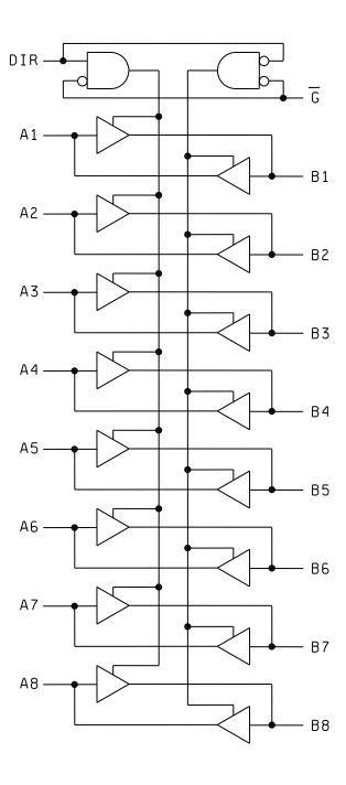
FIGURE 3. Logic diagrams.
