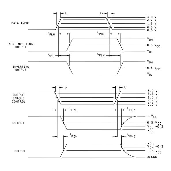
FIGURE 5. Switching waveforms and test circuit.
