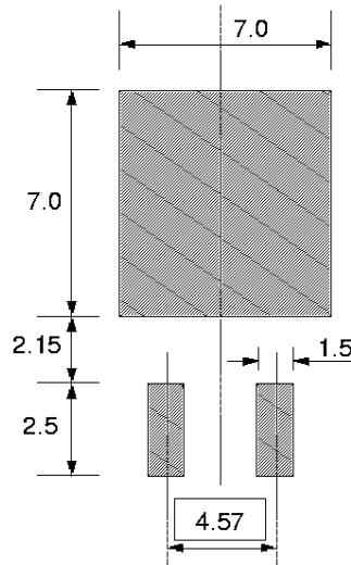
Fig.14. SOT428 : minimum pad sizes for surface mounting.
