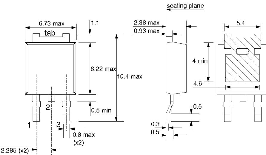
Fig.13. SOT428 : centre pin connected to tab.
