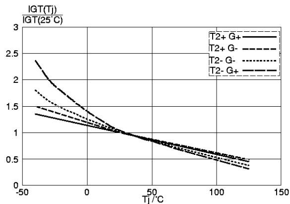
Fig. 7. Normalised gate trigger current
