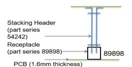
OAL = Distance between the two PCB – 2,4mm Example with PCB distance of 25mm : OAL = 25mm – 2,4mm = 22,6mm
