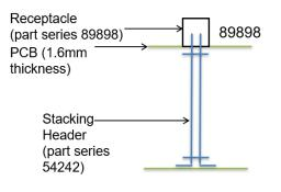
OAL = Distance between the two PCB + PCB thickness + 6,8mm *Example with PCB distance of 25mm :*OAL = 25mm + 1,6mm + 6,8mm = 33,4mm
