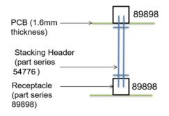
OAL = Distance between the two PCB – 2,4mm + PCB thickness + 7,1mm
