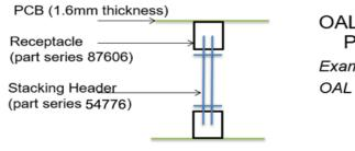
OAL = Distance between the two PCB – 7,4mm Example with PCB distance of 25mm : OAL = 25mm – 7,4mm = 17,6mm
