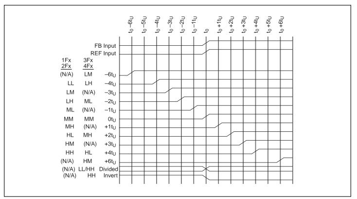
Figure 1. Typical Outputs with FB Connected to a Zero-Skew Output<sup>(3)</sup>
