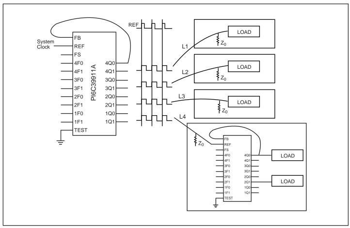
Figure 8. Board-to-Board Clock Distribution
