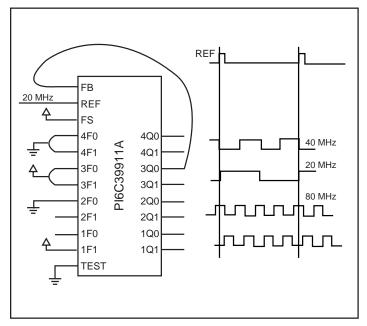
Figure 5. Frequency Multiplier with Skew Connections
