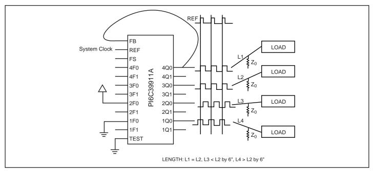
Figure 3. Programmable Skew Clock Driver
