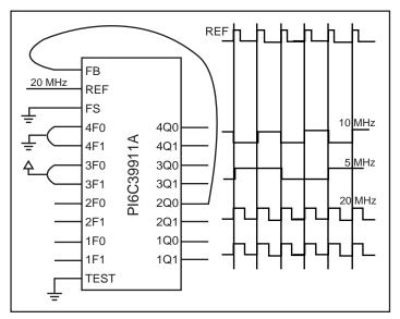
Figure 6. Frequency Divider Connections
