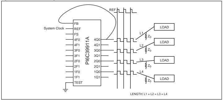
Figure 2. Zero-Skew and/or Zero-Delay Clock Driver
