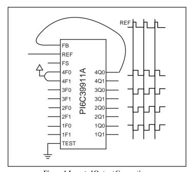
$Figure \, 4. \, Inverted \, Output \, Connections$
