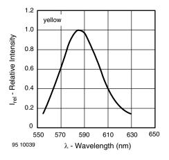
Fig. 9 - Relative Intensity vs. Wavelength
