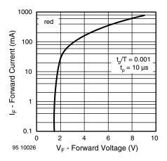
Fig. 5 - Forward Current vs. Forward Voltage
