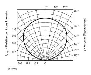
Fig. 3 - Relative Luminous Intensity vs. Angular Displacement
