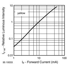
Fig. 11 - Relative Luminous Intensity vs. Forward Current
