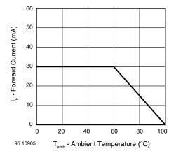
Fig. 1 - Forward Current vs. Ambient Temperature
