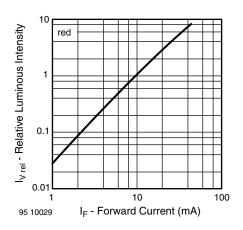
Fig. 6 - Relative Luminous Intensity vs. Forward Current
