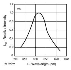
Fig. 4 - Relative Intensity vs. Wavelength
