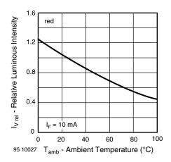
Fig. 8 - Relative Luminous Intensity vs. Ambient Temperature
