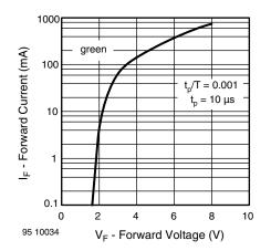
Fig. 15 - Forward Current vs. Forward Voltage
