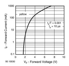
Fig. 10 - Forward Current vs. Forward Voltage
