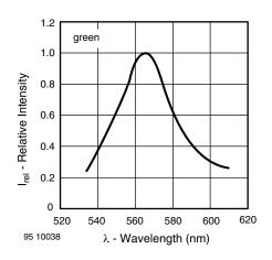
Fig. 14 - Relative Intensity vs. Wavelength
