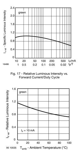
Fig. 18 - Relative Luminous Intensity vs. Ambient Temperature
