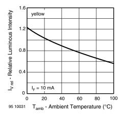
Fig. 13 - Relative Luminous Intensity vs. Ambient Temperature
