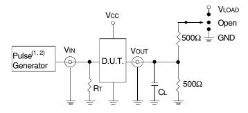
Test Circuits for All Outputs
