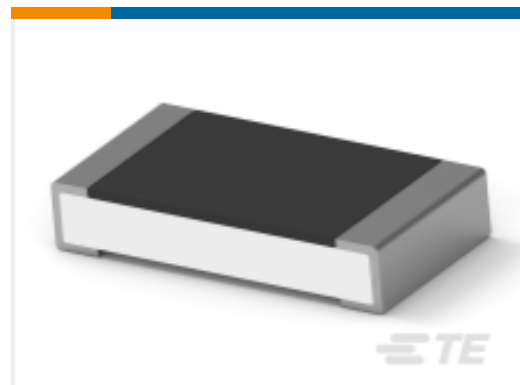
TE Part #4-2176391-7 RQ 1206 37K4 0.1% 10PPM 5K RL
