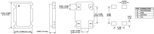
\*\*\*note: A 0.01  $\mu$ F bypass capacitor should be placed between  $V_{DD}$  (Pin4) and GND (Pin2) to minimize power supply line noise
