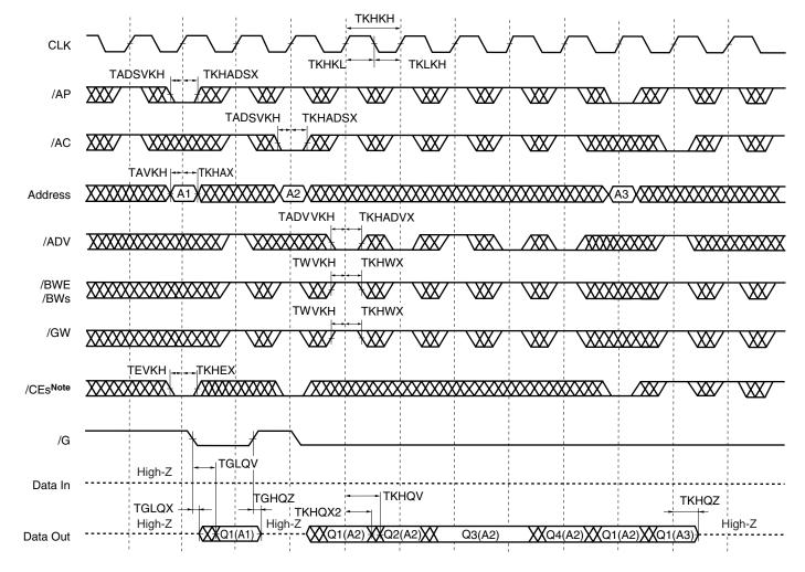
Note /CEs refers to /CE, CE2 and /CE2. When /CEs is LOW, /CE and /CE2 are LOW and CE2 is HIGH. When /CEs is HIGH, /CE and /CE2 are HIGH and CE2 is LOW.
