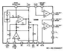
The low initial error allows the AD688 to be used as a system reference in precision measurement applications requiring 12-bit absolute accuracy. In such systems, the AD688 can provide a known voltage for system calibration and the cost of periodic recalibration can therefore be eliminated. Furthermore, the mechanical instability of a trimming potentiometer and the potential for improper calibration can be eliminated by using the AD688 and calibration software.
