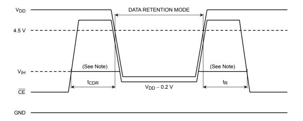
Note: When  $\overline{\text{CE}}$  is operating at the VIH level (2.4 V), the standby current is given by IDDS1 during the transition of VDD from 4.5 to 2.6 V.
