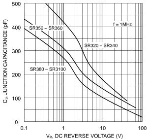
Fig. 5 Typical Junction Capacitance
