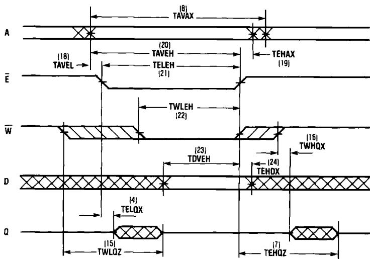
NOTE: In this mode,  $\bar{W}$  rises after  $\bar{E}$ . If  $\bar{W}$  falls before  $\bar{E}$  by a time exceeding  $TWLQZ$  (Max) -  $TELOX$  (Min), and rises after  $\bar{E}$  by a time exceeding  $TEHQZ$  (Max) -  $TWHQZ$  (Min), then Q will remain in the high impedance state throughout the cycle.
