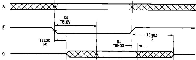
NOTE:  $\bar{W}$  is held high for entire cycle and D is ignored. Address is stable by the time  $\bar{E}$  goes low and remains valid until  $\bar{E}$  goes high.
