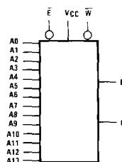
A — Address Input      D — Data Input
