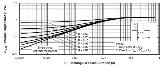
Fig. 4 - Maximum Thermal Impedance Z<sub>thJC</sub> Characteristics
