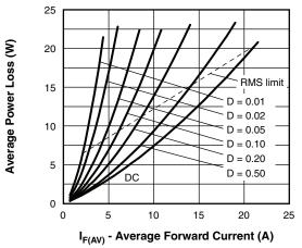
Fig. 6 - Forward Power Loss Characteristics
