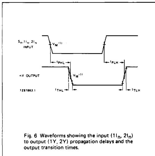
Fig. 6 Waveforms showing the input ( $11_n$ ,  $21_n$ ) to output ( $1Y$ ,  $2Y$ ) propagation delays and the output transition times.
