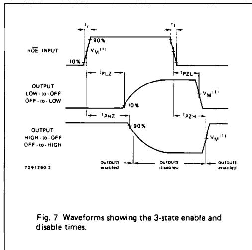
Fig. 7 Waveforms showing the 3-state enable and disable times.
